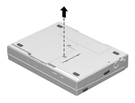
Figure 5-10. Removing the Hard Drive Security Screw
